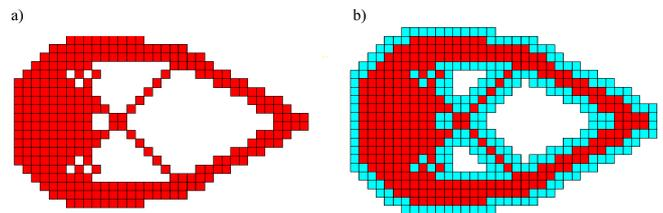
Fig. 2. The layer expansion algorithm: a structure before (a) and after operation of adding a layer of finite elements to the structure boundary (b)
