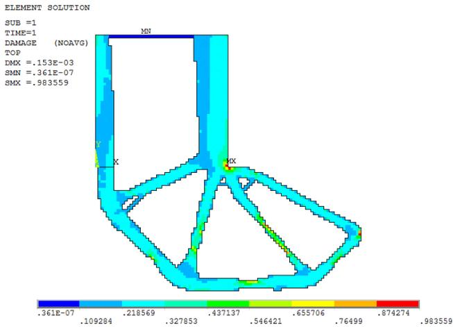
Fig. 8. The topology optimization result for multi-constraint (Dang Van and von Mises),  $\bar{g}_n = 1$ ;  $F = 30.8\%$
