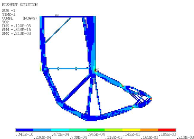
Fig. 11. The topology optimization result of the compliance constraint,  $\bar{g}_3 = 0.23e-3$ ;  $F = 23.4\%$
