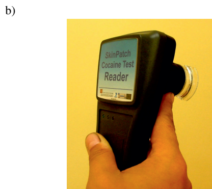
Fig. 13. Lab-on-a-paper – based test for detection of cocaine: a) scheme of the measurement setup for, b) view of the hand-held reader co-working with the test
