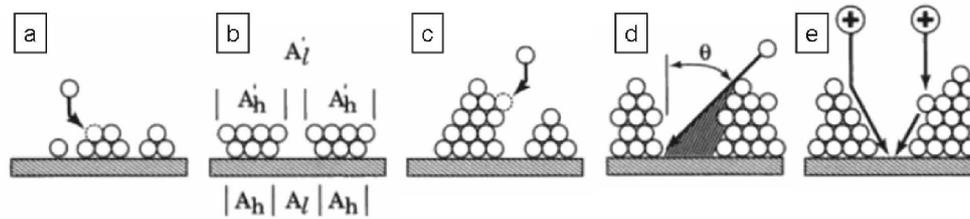
Fig. 5. Atomistic processes in quenched-growth structure development: (a) ballistic aggregation, (b) finite-size effect, (c) sideways attraction, (d) oblique shadowing, (e) void-filling by energetic particles (adapted from Ref. 11)
