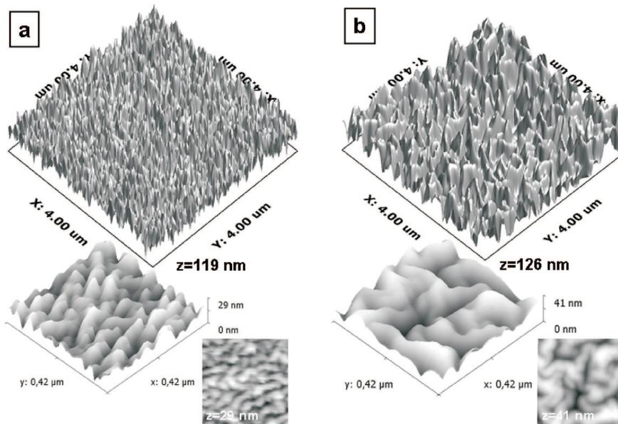
Fig. 7. AFM images of nucleation and growth structures of 20 nm thick PLD Ti coatings on PC a) and PU surfaces b), which are shown uncoated in Fig. 3a and c, respectively. The details of  $\sim 400 \times 400 \text{ nm}^2$  large areas show the nanostructure in two- and three-dimensional views
