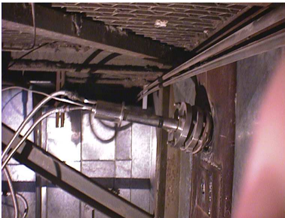
Fig. 5. The optical fibre probe with optoelectronic block
