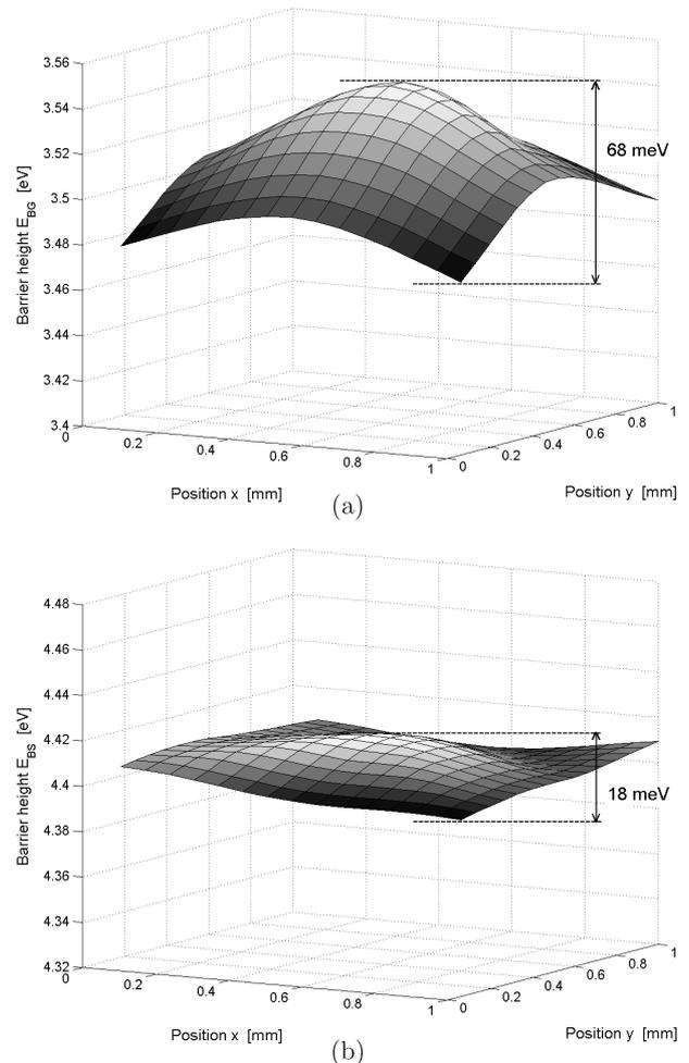
Fig. 9. Averaged two-dimensional distribution of a)  $E_{BG}$  and b)  $E_{BS}$  barrier heights measured using modified Powell-Berglund method for 26 MOS structures. Average  $E_{BG}$  and  $E_{BS}$  values were found for each of the 9 locations over the gate area (shown in Fig. 8) and used to determine distributions shown in the figure
