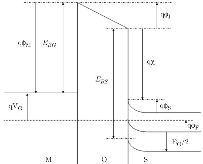
Fig. 4. Band diagram of the MOS system, at arbitrary gate potential  $V_G$ .  $E_{BG}$ ,  $E_{BS}$  are potential barrier heights at gate-dielectric and semiconductor-dielectric interfaces, respectively
