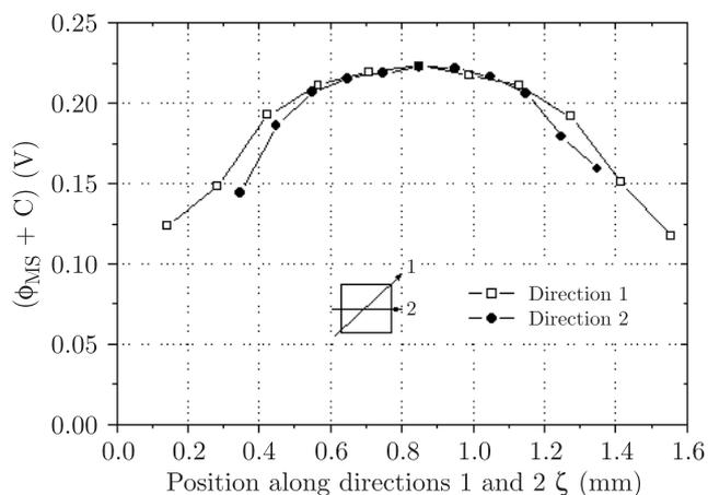
Fig. 1. Typical dependence of the  $(\phi_{MS} + C)$  voltage measured at the wavelength  $\lambda = 244$  nm on the position in Al-SiO<sub>2</sub>-Si(n<sup>+</sup>) structures with aluminum gate thickness  $t_{Al} = 35$  nm and SiO<sub>2</sub> layer thickness  $t_{OX} = 60$  nm. The direction is either (1) along the diagonal of the square gate, or (2) through the centre of the square gate and parallel to its edges
