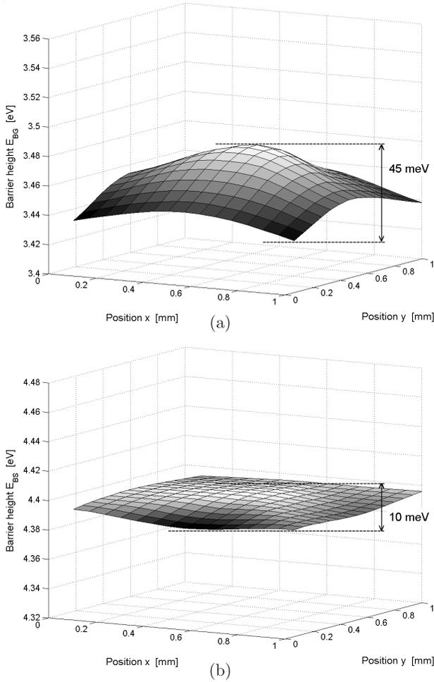
Fig. 10. Averaged two-dimensional distribution of a)  $E_{BG}$  and b)  $E_{BS}$  barrier heights measured using modified Fowler method for 26 MOS structures. Average  $E_{BG}$  and  $E_{BS}$  values were found for each of the 9 locations over the gate area (shown in Fig. 8) and used to determine distributions shown in the figure
