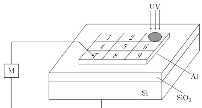
Fig. 8. The measurement system: the MOS structure with semitransparent Al gate is illuminated in 9 different locations over the gate area by a focused light beam. The photocurrent is measured in the external circuit  $M$
