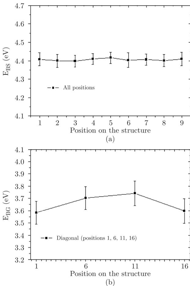
Fig. 14. Average values, shown by points connected by straight lines and standard deviations, shown by error bars, of local barrier height measurement results. a) Local  $E_{BS}$  measurement results for all the nine positions in the  $3 \times 3$  matrix over the gate area. b) Local  $E_{BG}$  measurement results in four positions lying on the diagonal of the  $4 \times 4$  matrix over the gate area
