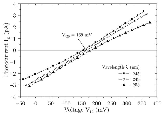
Fig. 7. The experimental characteristics  $I_P = f(V_G)$  taken for the  $V_{G0}$  voltage determination
