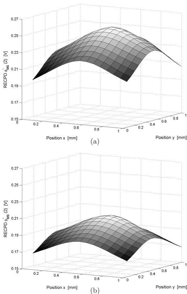
Fig. 12. Averaged two-dimensional distribution of  $\phi_{MS}^*(2)$  reduced effective contact potential difference calculated using  $E_{BG}$  and  $E_{BS}$  values determined by: a) the modified Powell-Berglund method and b) the modified Fowler method for 26 MOS structures. Average  $\phi_{MS}^*(2)$  values were found for each of the 9 locations over the gate area (shown in Fig. 8) and used to determine distributions shown in the figure
