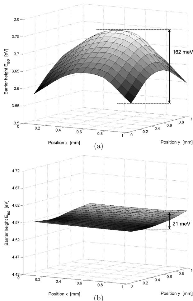
Fig. 13. Averaged two-dimensional distribution of (a)  $E_{BG}$  and (b)  $E_{BS}$  barrier heights measured using modified Powell-Berglund method for 30 MOS structures. Average  $E_{BG}$  and  $E_{BS}$  values were found for each of the 16 locations over the gate area and used to determine distributions shown in the figure
