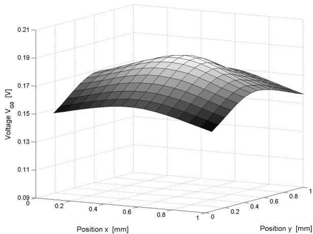
Fig. 11. Averaged two-dimensional distribution of  $V_{G0}$  values measured for 26 MOS structures. Average  $V_{G0}$  values were found for each of the 9 locations over the gate area (shown in Fig. 8) and used to determine the distribution shown in the figure
